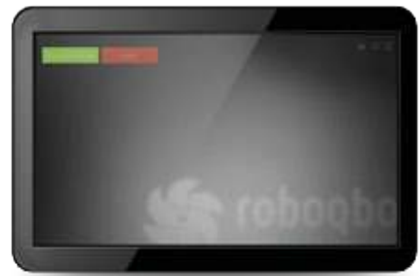
Screen size: 10.1" - Resolution: 1280 x 800px Connectivity: USB - Ethernet (LAN) - Wireless LAN (*optional)
